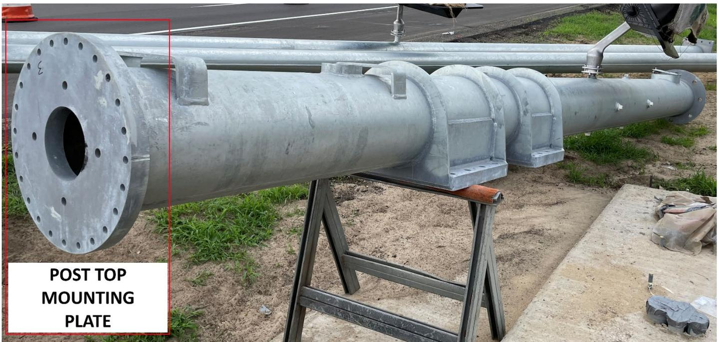
The design of the TS post top plate to provide rotation for the extension was a continuation of functionality that
