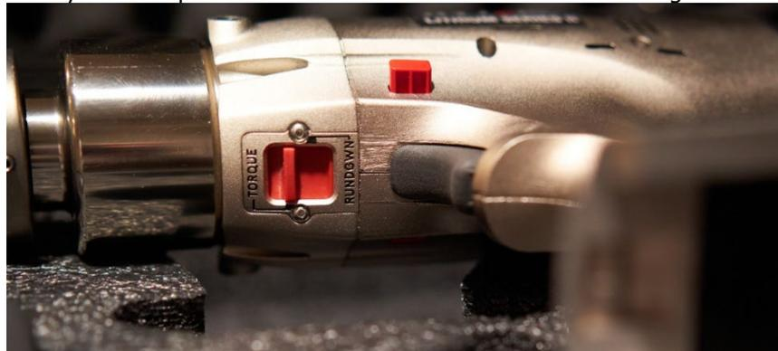
Due to the vast differences in the torque required for applications ranging from high strength bolts to large anchor rods in TS poles it is impossible for a single electric torque tool to cover such a broad range of sizes and torque specifications. For tasks involving a wide array of bolt and anchor rod sizes, TS pole installers typically need to invest in a series of torque wrenches to properly address the diverse torque requirements of different projects.
